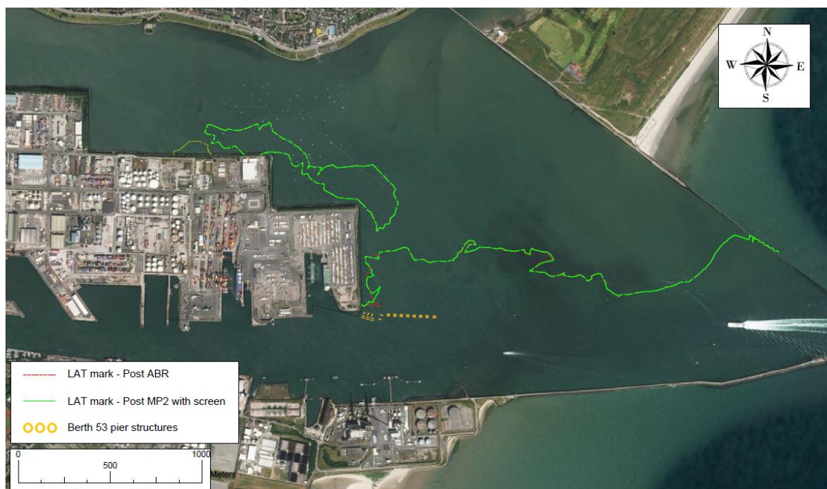
Figure 5.28 Position of the Lowest Astronomical Tide mark post ABR (red line) and post MP2 with the thruster screen in situ (green line).
